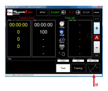
When the test is completed, it will be necessary to back up the generated Files. Press the button 17 to access the GRAPHICS screen which will generate TWO performed Test back up files.
